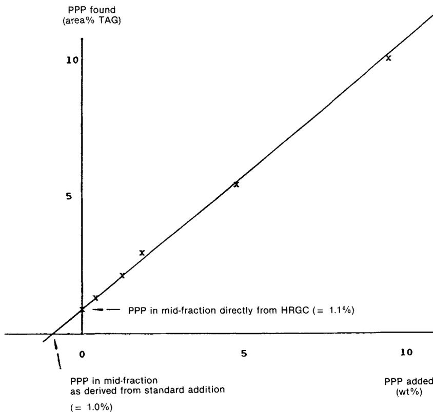
FIG. 3. Linearity of response and quantitative accuracy for PPP (15 m  $\times$  0.53 mm i.d. methyl 65%-phenyl wide-bore capillary column. Abbreviations: P = palmitic acid; TAG, triacylglycerols; HRGC, high-resolution gas chromatography.
