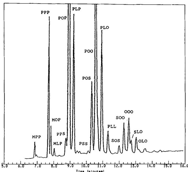
FIG. 2. Palm oil: 15 m  $\times$  0.25 mm i.d. methyl 65%-phenyl wide-bore capillary column; 350–360°C @ 1°C/min. Abbreviations: M, P, O, L, S = myristic, palmitic, oleic, linoleic and stearic acids, respectively.
