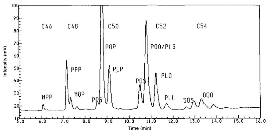
FIG. 1. Palm oil: 15 m  $\times$  0.53 mm i.d. methyl 65%-phenyl wide-bore capillary column; 345–365°C @ 1°C/min. Abbreviations: M, P, O, S, L = myristic, palmitic, oleic, stearic and linoleic acids, respectively.
